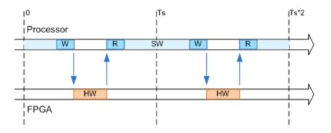
The shaded areas indicate when the processor and FPGA are running. During each sample time, the processor writes to the FPGA, then stops and waits for an indication that the FPGA has finished processing before continuing to run. Each time the FPGA runs, it executes the logic generated for one DUT subsystem sample time.
