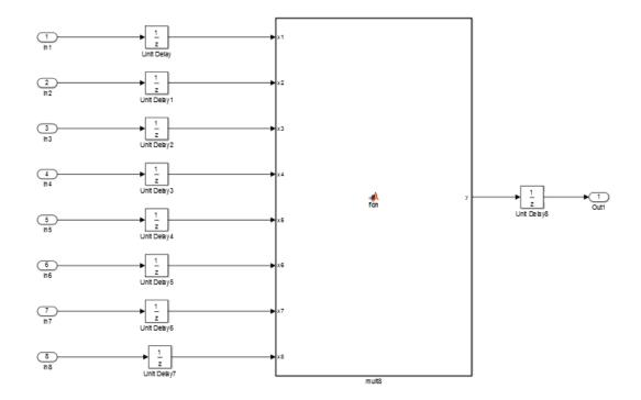
The following shows a chain of multiplications as coded in the mult8 MATLAB Function block:
