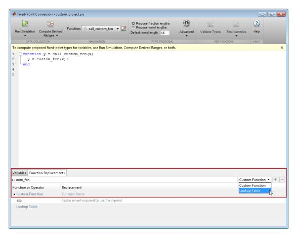
The tool adds custom\_fcn to the list of functions that it will replace with a Lookup Table. By default, the lookup table uses linear interpolation, 1000 points, and the design minimum and maximum values that the app detects by either running a simulation or computing derived ranges.
