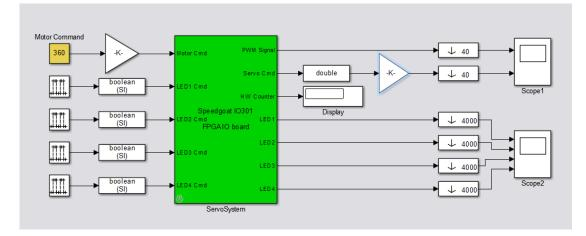
The model contains the Simulink Real-Time interface subsystem. This new subsystem replaces the DUT (ServoSystem) in the original model. It replaces the internals of the original DUT with a Simulink Real-Time FPGA block and other blocks to work with the algorithm on the FPGA.
