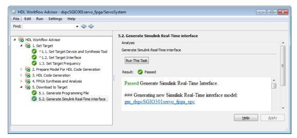
4 The **Result** pane displays a link to a generated model — gm\_dxpcSGI0301servo\_fpga\_xpc. Click the link to open the model.
