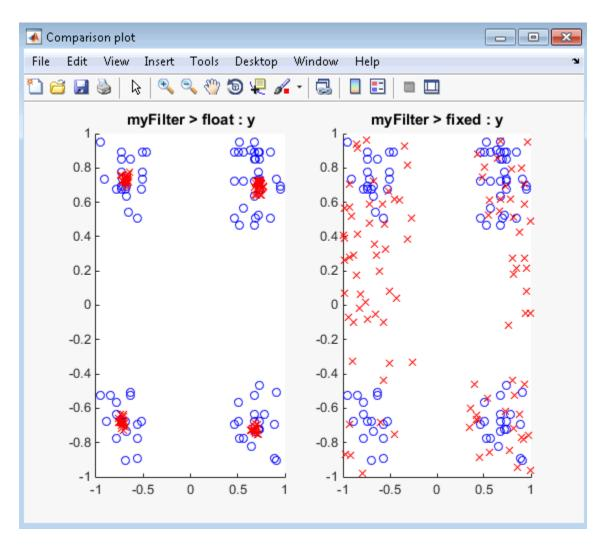
The plot shows that the fixed-point results do not closely match the floating-point results. Increase the word length to 24 and then convert to fixed point again.
