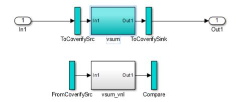
The vsum subsystem has been highlighted in cyan. This highlighting indicates that the subsystem differs in some respect from the vsum subsystem of the original model.
