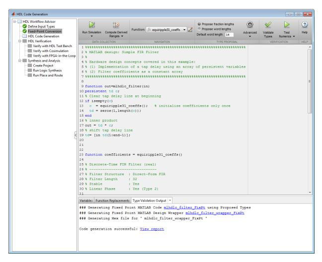
Click the links to the generated code in the Workflow Advisor log window to examine the generated fixed-point design, wrapper, and test bench.
