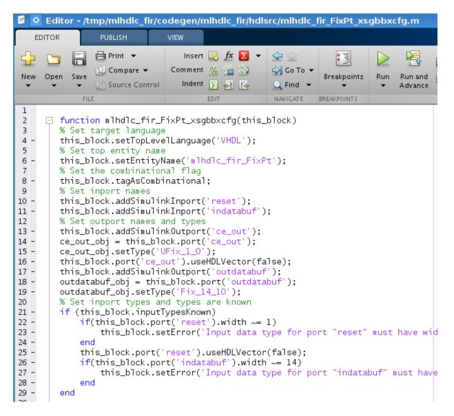
You can now use the generated Xilinx System Generator Black Box block and configuration file in a larger system design.
