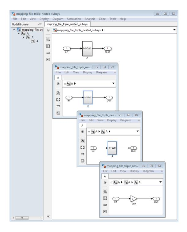
When code is generated for the top-level subsystem A, makehdl works its way up from the deepest level of the model hierarchy, generating unique entity names for each subsystem.
