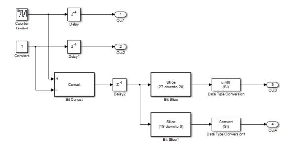
The Delay and Delay1 blocks merge and map to a dual-port RAM in the generated HDL code by satisfying the following conditions:
