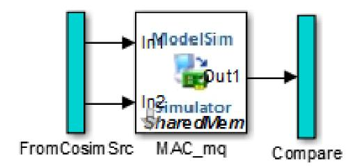
The FromCosimSrc subsystem receives the same input signals that drive the DUT. In the gm\_hdl\_cosim\_demo1\_mq0 model, the subsystem simply passes the inputs on to the HDL Cosimulation block. Signals of some other data types require further processing at this stage (see "Signal Routing Between Simulation and Cosimulation Paths" on page 17-45).
