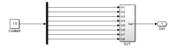
The top-level subsystem is the design under test (DUT). The DUT subsystem contains one subsystem, subsys, and other blocks.
