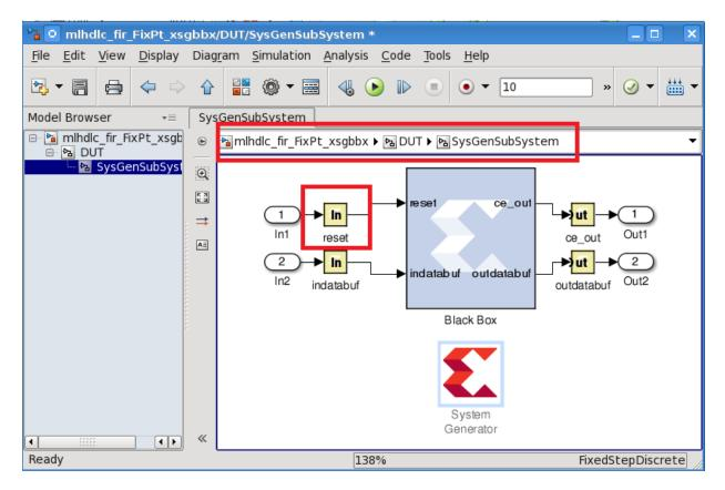
Notice that in addition to the data ports, there is a reset port on the black box interface, while 'clk' and 'ce' are registered to System Generator by the Black Box configuration file.
