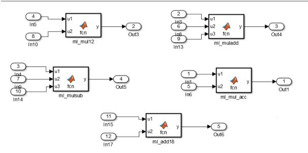
For example, the ml\_mul\_acc MATLAB Function block shows how to write a multiplyaccumulate operation in MATLAB. hdlfimath applies fixed-point math settings that are appropriate for HDL code generation.
