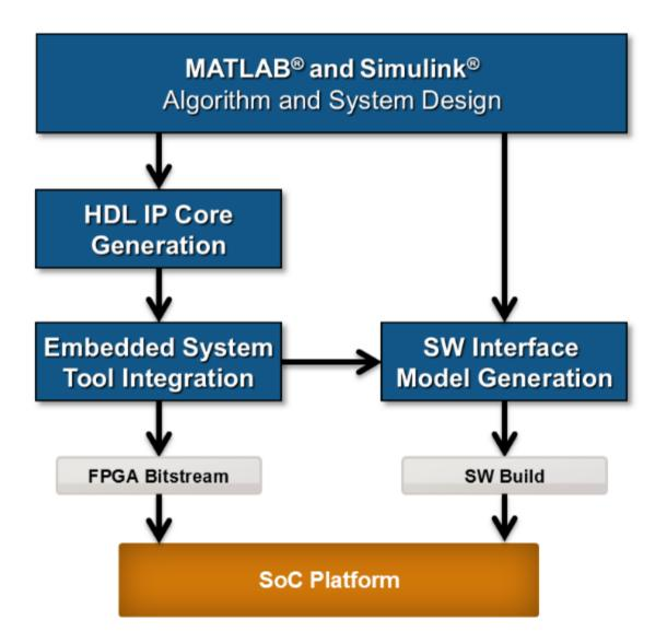
1 *MATLAB and Simulink Algorithm and System Design*: You begin by implementing your design in MATLAB or Simulink. When the design behavior meets your requirements, decide how to partition your design: which parts you want to run in hardware, and which parts you want to run in embedded software.
