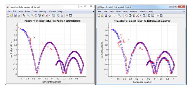
Having chosen comparison plots option you will see additional plots that compare the floating and fixed point simulation results for each output variable.
