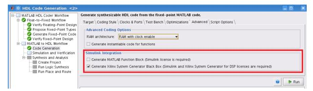
To generate code compatible with a Xilinx System Generator Black Box, set:
