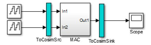
The two subsystems labelled ToCosimSrc and ToCosimSink do not change the performance of the simulation path. Their purpose is to capture stimulus and response signals of the DUT and route them to and from the HDL cosimulation block (see "Signal Routing Between Simulation and Cosimulation Paths" on page 17-45).
